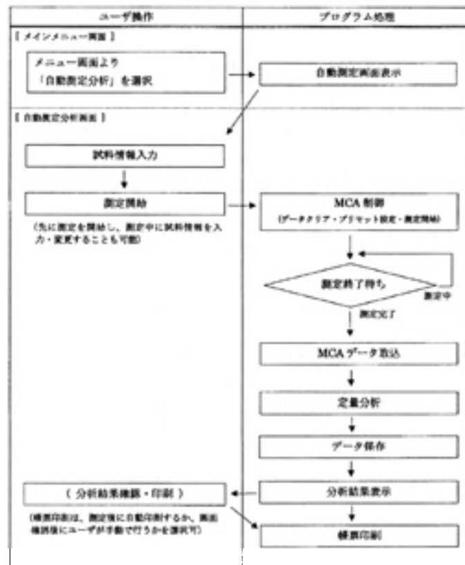
Fig.4 Analytical procedure for NAI scintillation counter, CAN-OSP-NAI, Aloka Co.
