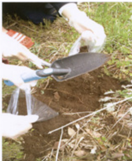
Fig.2 The soil sample collected in the field area. The hands covered with polyethylene globe, which gives a protection from radioactive nuclides.
