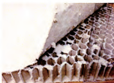
Fig.3 Cardboard honeycomb panel
