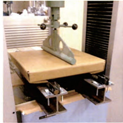
Fig.17 Hydraulic system universal testing machine and cardboard ATCP
