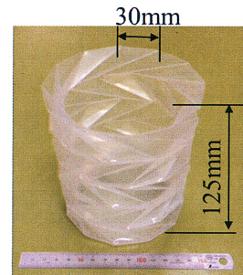
Fig. 4 The prototype product of foldable cylindrical structure based 12 square type with 150mm scale
