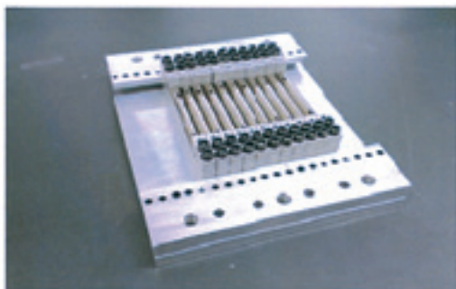
Fig.4 Actual measuring stand of Halbach array arranged eleven holders with cylinder shaped permanent magnets.
