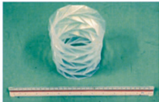
Fig. 3 The prototype product of foldable cylindrical structure based 12 square type with 300mm scale
