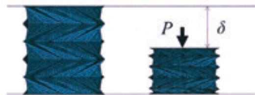
(c) Deformation simulation by FEM analysis
