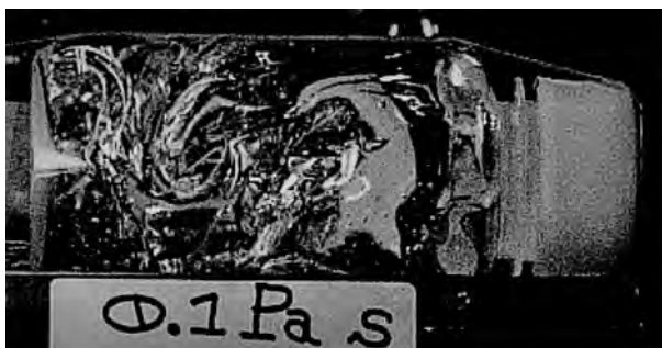
Fig. 4 Snapshot of the shaken plastic bottle containing liquid of the viscosity of 1 \times 10^{-1} Pa s. The frequency and amplitude are 3.0 Hz and 6 \times 10^{-2} m, respectively.
