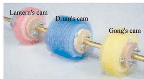
Fig. 11 Cam block of three robots that were fixed in rotating shaft.
